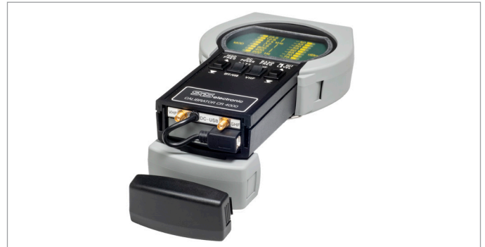
Connection options on the underside of the CR 4000
